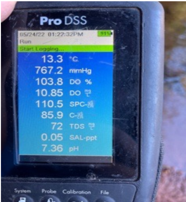
Figure 5. YSI Pro DSS © water quality sampler. Parameters from top to bottom include, Temperature (°C), Barometer (mmHg), Dissolved Oxygen % (DO%), Dissolved Oxygen mg/l (DO mg/L), Specific Conductivity (SPC uS/cm), Conductivity (C-uS/cm), Total Dissolved Solids (TDS), Salinity (in parts per thousand) and pH.
