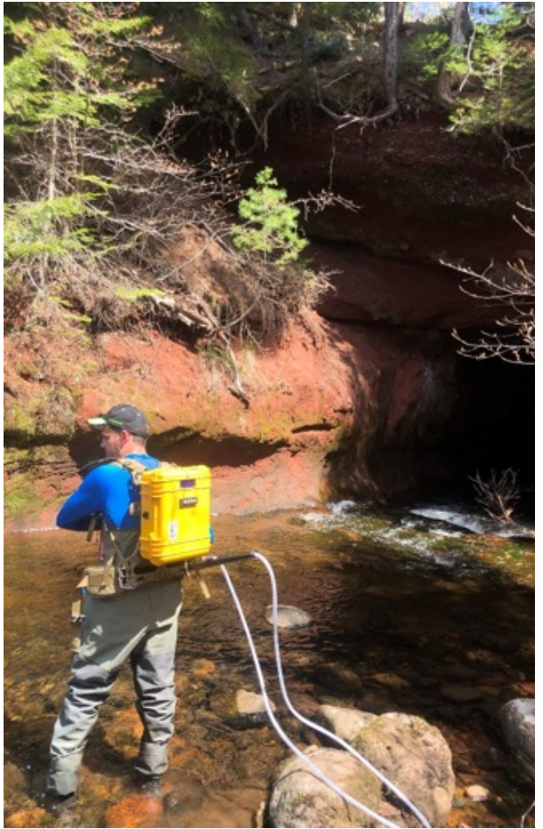
Figure 6. In-river DNA collection via OSMOS eDNA sampler backpack.
